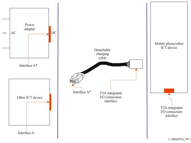
NOTE - Interface A\* is not always necessarily physically separated.
