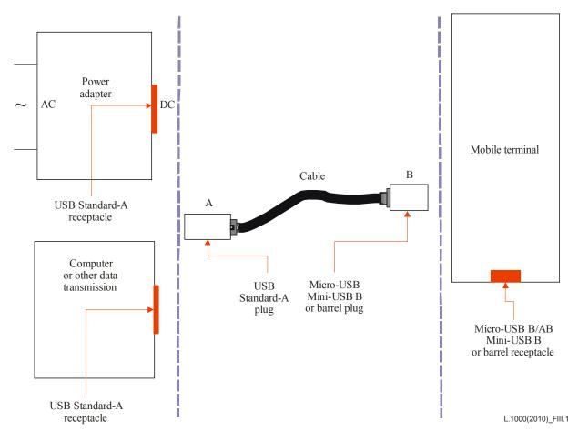
**Figure III.1 – Basic architecture**
