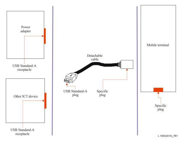
Figure B.1 – Basic elements of universal charger solution for mobile terminals
