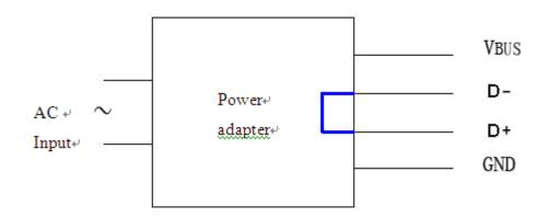
Figure III.2 – The D+ and D– signal line in the power adapter
