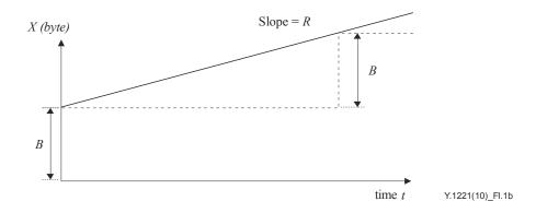
Figure I.1b – Single rate, single bucket size token bucket – 'worst-case' bursty flow
