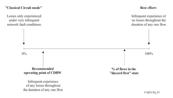
Figure 1 – CDBW transition from a best effort service to imperceptibly near a "circuit mode" service
