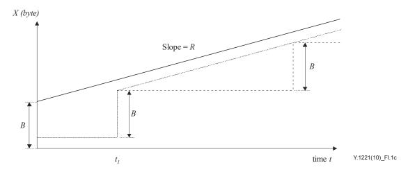
Figure I.1c – Single rate, single bucket size token bucket – 'worst-case' flows after inactivity
