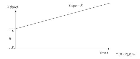
Figure I.1a – Single rate, single bucket size token bucket – 'worst-case' flow
