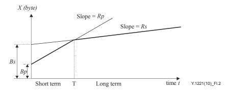
Figure I.2 – Two rates, two token buckets (Bp < Bs) – 'worst-case' flow
