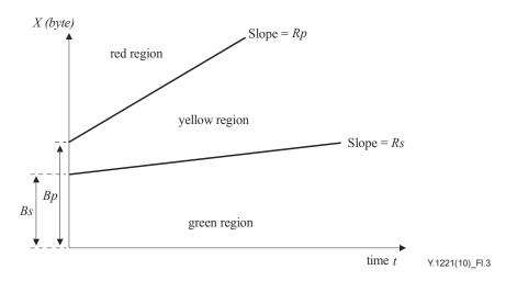
Figure I.3 – Two rates, two token bucket (Bp > Bs) – 'worst-case' flow
