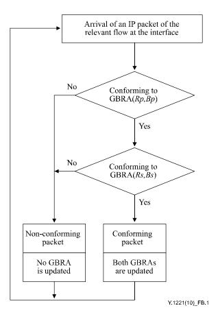
Figure B.1 – Behaviour of two coordinated generic byte rate algorithms
