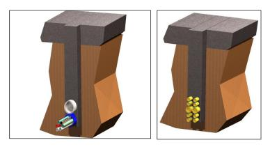
Figure 1 – Examples of urban-trenching duct installation configuration
