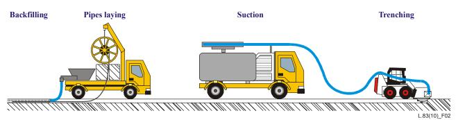
Figure 2 – Daily reduced trenching technique logical scheme
