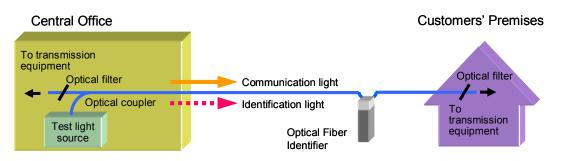
Figure I.1 – Configuration of optical fibre identification
