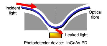
Figure 2 – Typical configuration of bent part of optical fibre identifier
