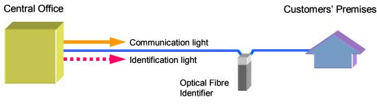
Figure 1 – Configuration for optical fibre identification
