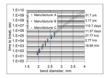
Figure I.1 – Results of 2-point bend static fatigue tests for optical fibres from three manufacturers Solid lines denote extrapolation of average from the experimental data [b-Mazzarese]
