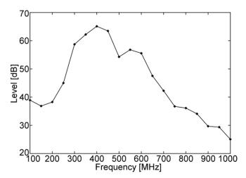
Figure III.3 – Measurement results for SN at each receiving frequency band in radiated electromagnetic interference
