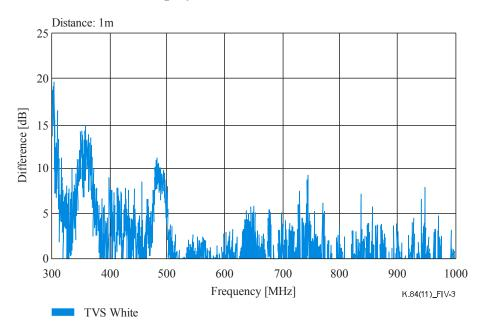
Figure IV.3 – Difference in levels of spectrum when white and TVS images are displayed from 300 to 1000 MHz
