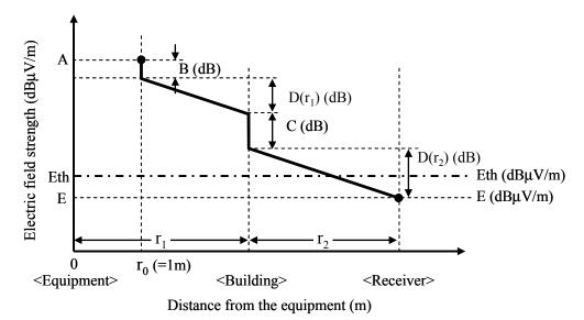
**Figure 5.3-2** – Attenuation emission from the equipment
