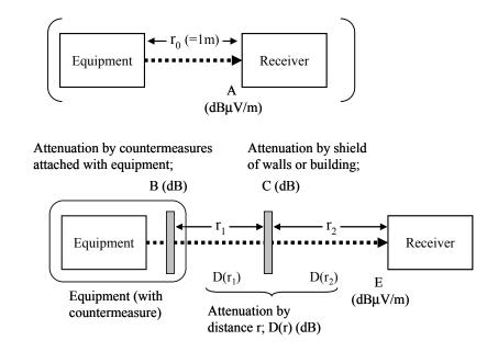
**Figure 5.3-1** – Attenuation of emission from equipment
