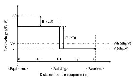
Figure 5.4-1 – Levels for conducted emission from the equipment
