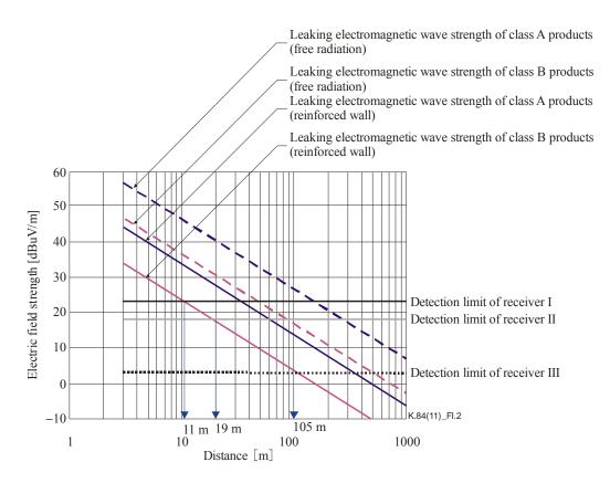
Figure I.2 – Relationship between possible electric field strength (strength of leaking information) and distance for EMSEC
