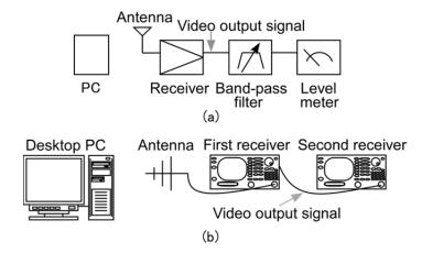
Figure III.2 – (a) System block configuration and (b) measurement system to detect information signal in radiated electromagnetic emissions of PC
