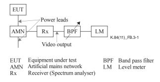
Figure B.3-1 – Test configuration for receivers
