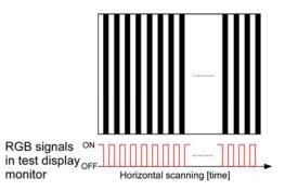
Figure III.1 – Test image with periodic 8-pixel wide vertical stripes
