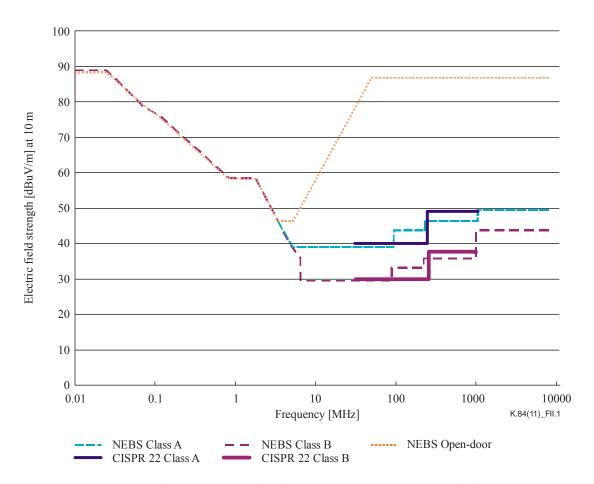
Figure II.1 – Comparison of reference emission values ([CISPR 22] and [b-NEBS GR 1089])
