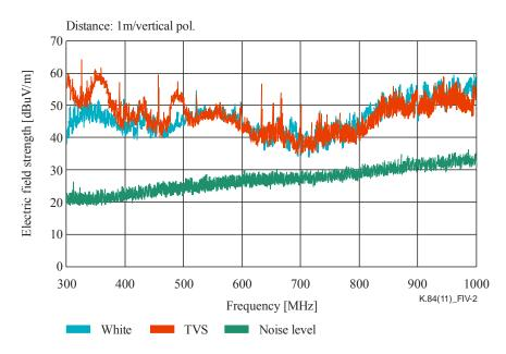
Figure IV.2 – Received level when white and TVS images are displayed from 300 to 1000 MHz
