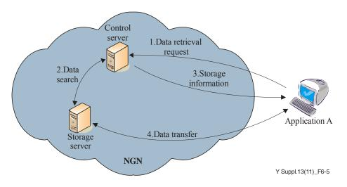
**Figure 6-5** – providing user information to applications
