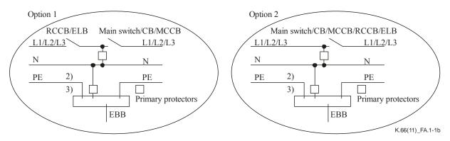
NOTE 5 – The SPD may be installed before the ELB (option 1) or after the ELB (option 2). If option 2 is used, nuisance tripping of the circuit breaker may occur, particularly if it contains an RCD.
