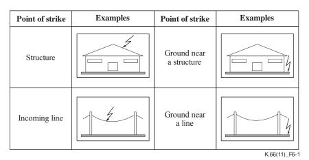
Figure 6-1 – Examples of direct and indirect lightning to the customer's building and services
