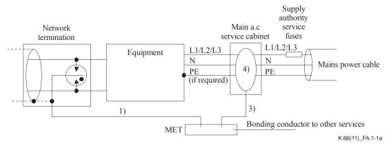
NOTE 1 – Total length of bonding wire to MET should be as short as possible (< 1.5 m if there is a significant risk of a direct lightning strike).
