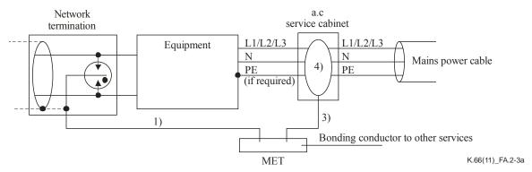
NOTE 1 – Total length of bonding wire to MET should be as short as possible (< 1.5 m if there is a significant risk of a direct lightning strike).
