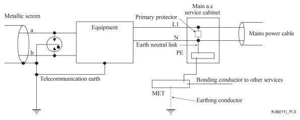
NOTE 1-An earth electrode is not required at the customer's premises in all power systems, it may be supplied in the distribution network.
