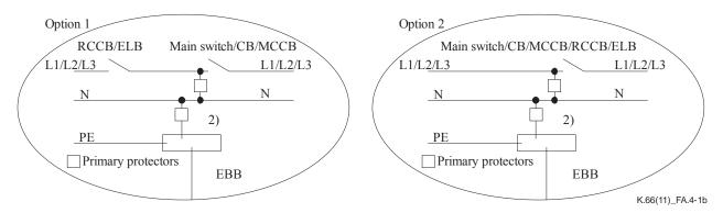
NOTE 5 – The SPD may be installed before the ELB (option 1) or after the ELB (option 2). If option 2 is used, nuisance tripping of the circuit breaker may occur, particularly if it contains an RCD.
