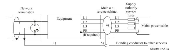
NOTE 1 – Total length of bonding wire to MET should be as short as possible (< 1.5 m if there is a significant risk of a direct lightning strike).
