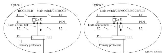
NOTE 5 – The SPD may be installed before the ELB (option 1) or after the ELB (option 2). If option 2 is used, nuisance tripping of the circuit breaker may occur, particularly if it contains an RCD.
