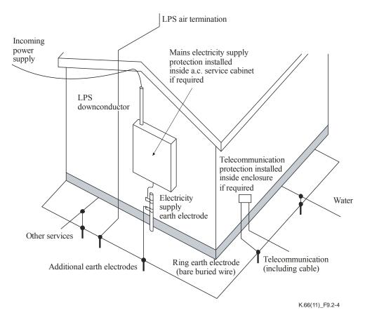
Figure 9.2-4 – Ring earth electrode
