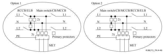
NOTE 6 – The SPD may be installed before the ELB (option 1) or after the ELB (option 2). If option 2 is used, nuisance tripping of the circuit breaker may occur, particularly if it contains an RCD.
