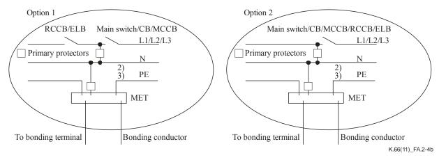
NOTE 6 – The SPD may be installed before the ELB (option 1) or after the ELB (option 2). If option 2 is used, nuisance tripping of the circuit breaker may occur, particularly if it contains an RCD.
