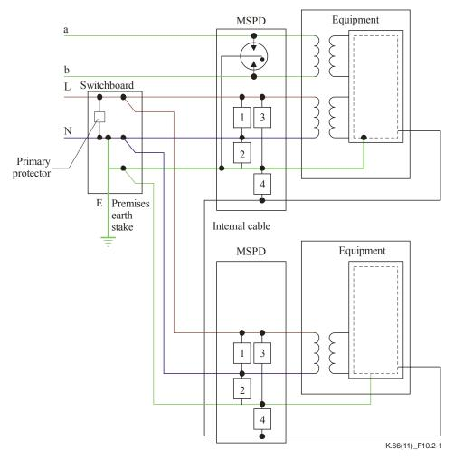
NOTE – SPDs 1, 2 and 3 need to be suitable for use on the mains. SPD 4 will need to be suitable to protect the equipment's internal port.
