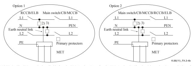
NOTE 6 – The SPD may be installed before the ELB (option 1) or after the ELB (option 2). If option 2 is used, nuisance tripping of the circuit breaker may occur, particularly if it contains an RCD.
