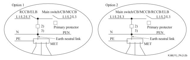
NOTE 6 – The SPD may be installed before the ELB (option 1) or after the ELB (option 2). If option 2 is used, nuisance tripping of the circuit breaker may occur, particularly if it contains an RCD.
