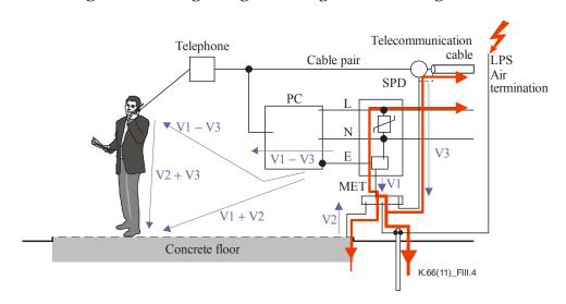
Figure III.4 – Lightning strike to structure
