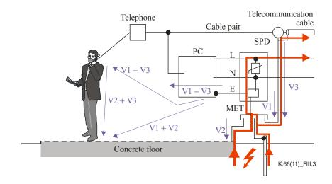
Figure III.3 – Lightning strike to ground resulting in EPR
