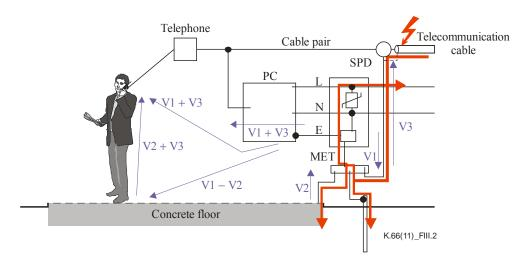
Figure III.2 – Lightning strike to the telecommunication cable
