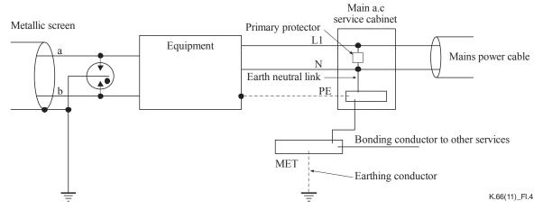
NOTE 1-An earth electrode is not required at the customer's premises in all power systems, it may be supplied in the distribution network.
