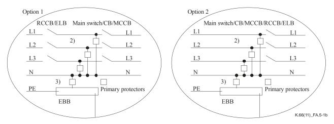
NOTE 5 – The SPD may be installed before the ELB (option 1) or after the ELB (option 2). If option 2 is used, nuisance tripping of the circuit breaker may occur, particularly if it contains an RCD.
