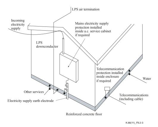
Figure 9.2-3 – Common bonding network (CBN)
