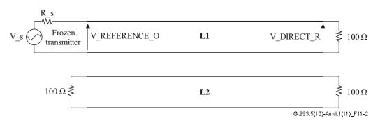
Figure 11-2 – Definition of downstream Xlin (direct channel received voltage)
