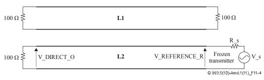
Figure 11-4 – Definition of upstream Xlin (direct channel received voltage)
