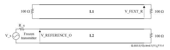
Figure 11-1 – Definition of downstream Xlin (FEXT channel received voltage)
