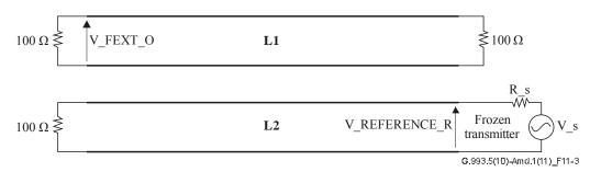
Figure 11-3 – Definition of upstream Xlin (FEXT channel received voltage)
