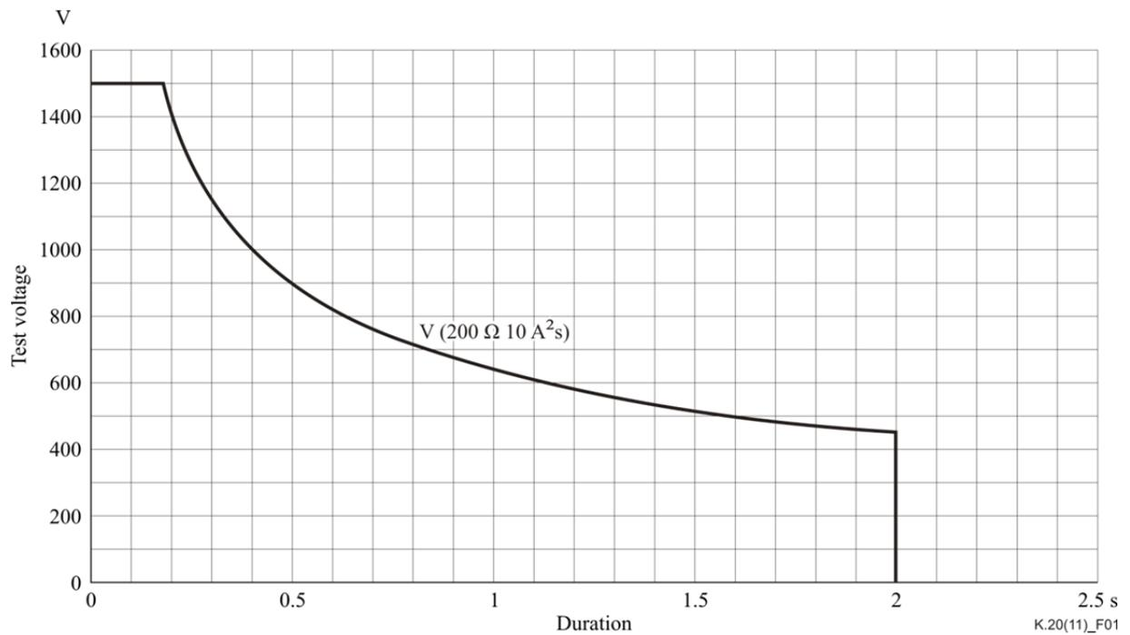
**Figure 1 – Test voltage versus duration to give 10 A<sup>2</sup>s with 200 Ω**
