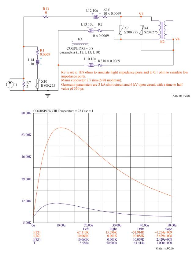
Figure C.2 – Simulation of an EPCOS B80K275 MOV primary protector with S20K275 MOVs in the MSPD
