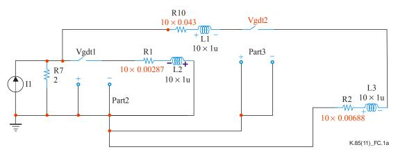
Mains conductor 2.5 mm (6.88 mohm/m) CLP bond conductor 6 mm<sup>2</sup> (2.87 mohm/m) Two conductors of 0.5 mm telecom conductor (43 mohm/m)
