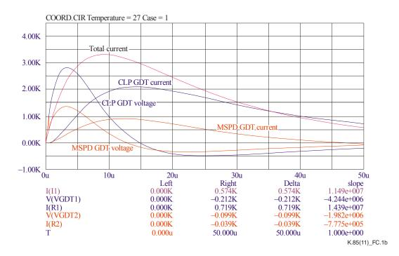
Figure C.1 – Simulation of a 10 m bond wire primary protector GDT with an MSPD connected to earth via 10 m of power earth wire
