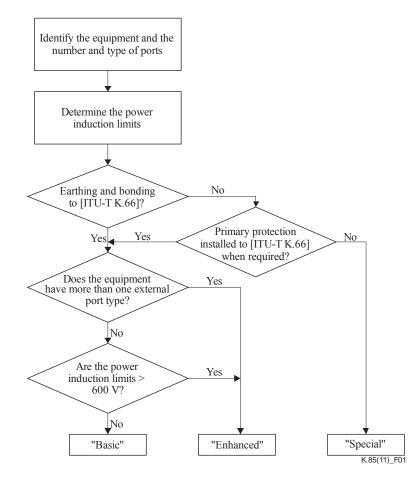
**Figure 1 – Flowchart for determining required level of resistibility**
