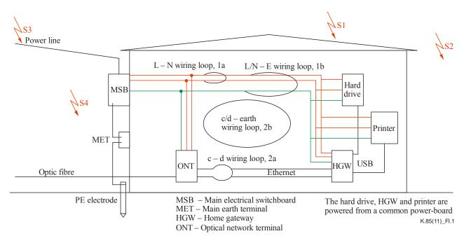
**Figure I.1 – Schematic of building wiring showing inductance loops**
