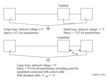
Figure II.3 – Induced voltage depends on the equipment type
