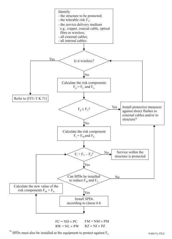
Figure D.2 – Procedure for selecting protection measures in a structure
