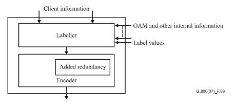
NOTE – A transport processing function may contain more than one labeller and encoder. The arrows external to the information system represent information that is presented via ports.
