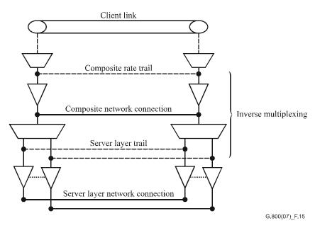
Figure 6-14 – Client link supported by inverse multiplexing
