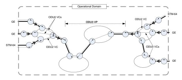
Figure V.3 – Example of virtual path (aggregation of service instances)
