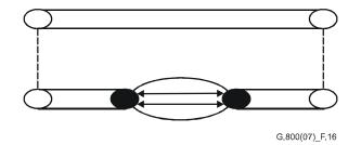
Figure 6-15 – Serial compound composed of component links and a subnetwork with configured subnetwork connections
