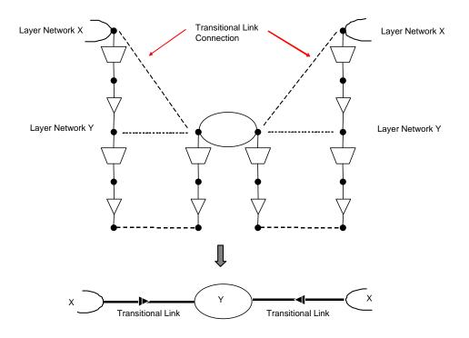
Figure 6-1 – Transitional link between layer networks X and Y
