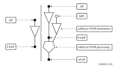
Figure 8-2 – Insertion at a forwarding end point
