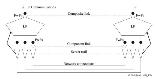
Figure 9-2 – Transport model for composite link (destination forwarding network)
