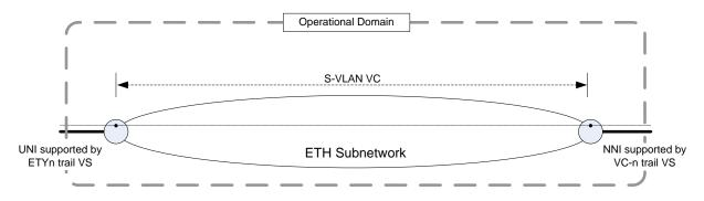
Figure V.1 – Example of virtual channel (transport-service instance)
