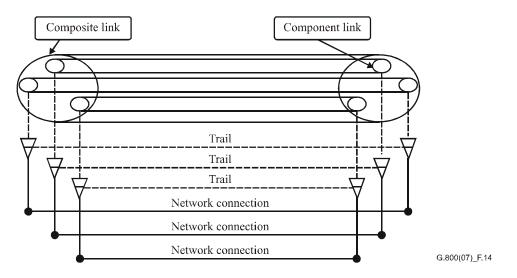
Figure 6-13 – Composite link supported by multiple independent server layer trails
