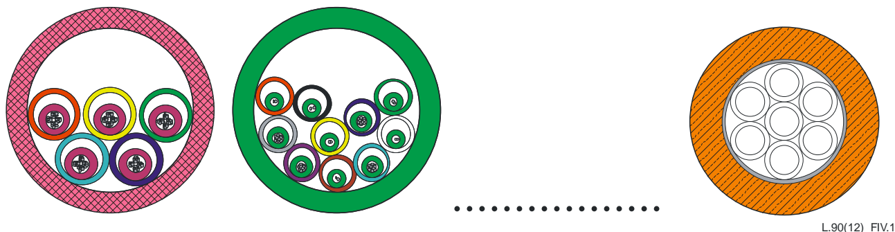
Figure IV.1 – Examples of loose bundles of mini-tubes (left and middle, for microcables with 24-60 and 2-24 optical fibres per mini-tube, respectively) and tight bundle of mini-tubes (right, for fibre members)
