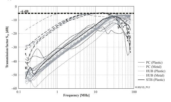
Figure I.2 – Measured transmission factors of IP-based communication devices
