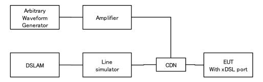
Figure 1 – Example block diagram of the test set-up
