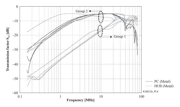
Figure I.4 – Transmission factors for devices with metal frames
