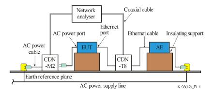
**Figure I.1 – Measurement set-up for transparency**
