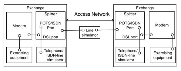
Figure A.1 – DSL access system configuration
