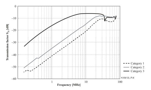
Figure I.8 – Transmission factors S<sub>21</sub> for three categorized models
