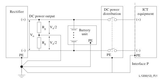
Figure I.1 – Example of the basic configuration of a grounding system for an 'up to 400 VDC' system
