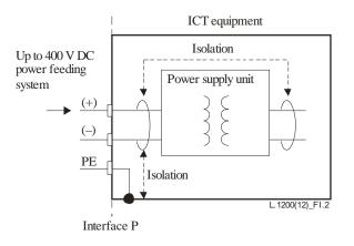
Figure I.2 – Grounding system configuration for an 'up to 400 VDC' system
