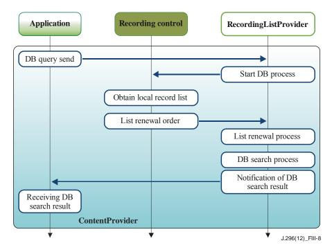
Figure III.8 – Sequence of content search for the content stored in the local storage
