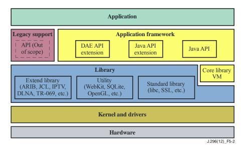
Figure 5-2 – Basic software architecture
