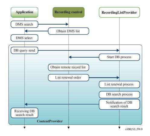
Figure III.9 – Sequence of content search for the content stored in the DMS connected to the home network
