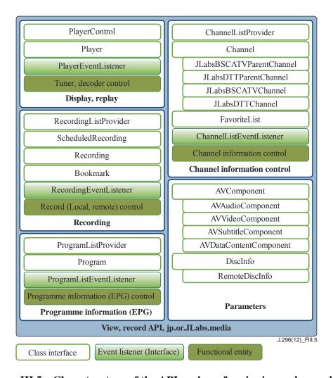
Figure III.5 – Class structure of the API package for viewing and recording
