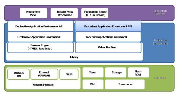
Figure III.1 – Relationship of the procedural application environment and other functions in the entire functional diagram
