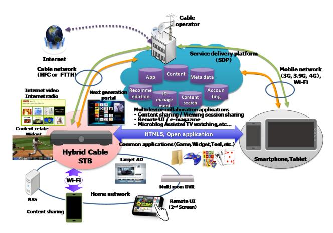
Figure 5-3 – Service delivery architecture
