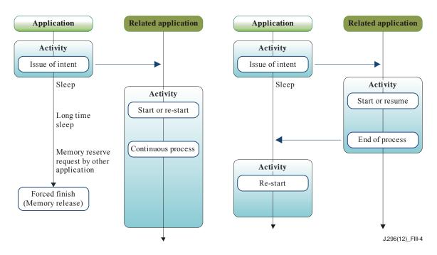
Figure III.4 – State transition diagram of the activity for Intent (left: one-way transition, right: both-way transition with suspend and resume)
