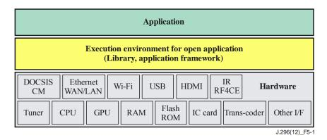
Figure 5-1 – Overall functional diagram
