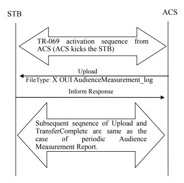
Figure A.3 – Measurement report sequence corresponding to the specific request
