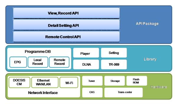
Figure III.2 – Relationship between the API package defined in this annex and other functions
