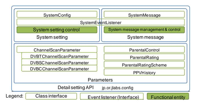
Figure III.10 - API class structure for detailed configuration
