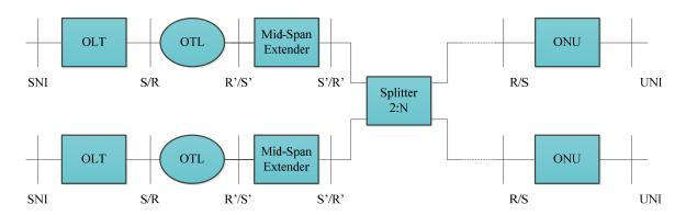
Figure 9 – Extended Type B protection architecture with two independent RE units
