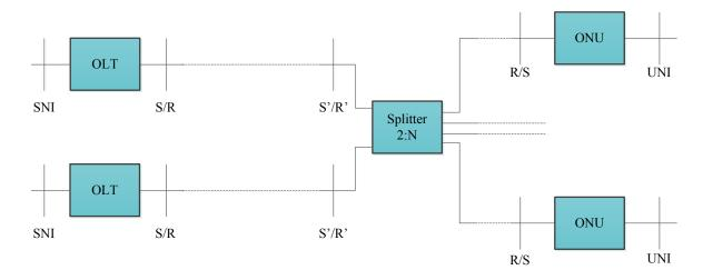
Figure 4 – Dual parented Type B protection
