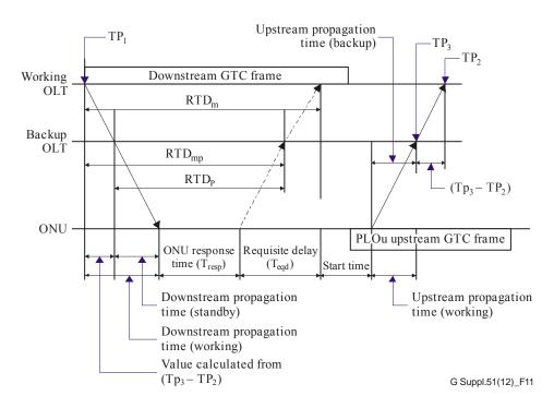
Figure 11 – Relationship between time references when the backup path is shorter than the working path
