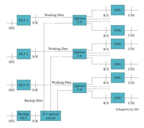
Figure 7 – Type B with N:1 using optical switch
