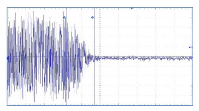
Figure 8 – Example trace of gradual loss of signal upon fibre cut
