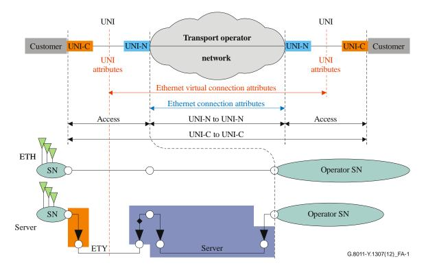
Figure A.1 – Single-provider view of Ethernet service areas with distributed UNI-N
