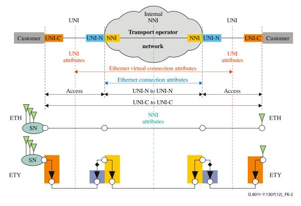
Figure 6-2 – Single-provider with NNI view of Ethernet service areas
