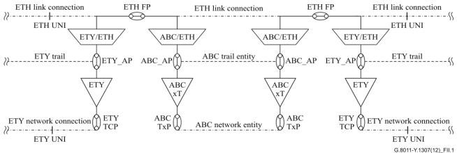
ABC - a connection-oriented circuit switched or connection-oriented packet switched or connectionless technology ABC - xT, x = T, connection-oriented trail termination for technology ABC ABC - xT, x = T, connection-oriented trail termination for technology ABC
