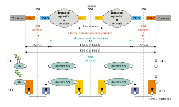
Figure 6-3 – Multi provider with NNI view of Ethernet service areas
