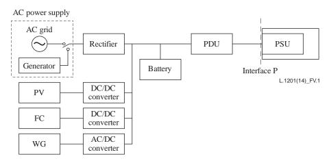
Figure V.1 – Direct connection in DC of PV, FC or WG generators to a DC power feeding
