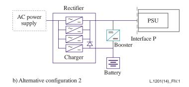
Figure IV.1 – Configurations of the rectifier/battery system
