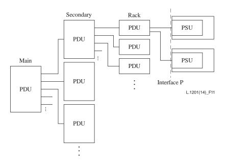
Figure 11 – Example configuration of a multi-level PDU
