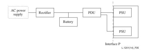
Figure 5 – System configuration with the redundant input of ICT equipment
