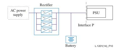
Figure 10 – Basic configuration of rectifier
