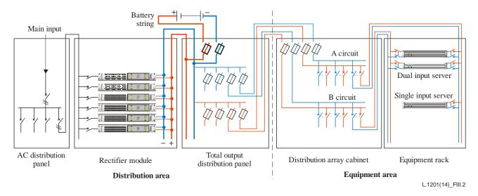
**Figure III.2** – **Two-level distribution structure**
