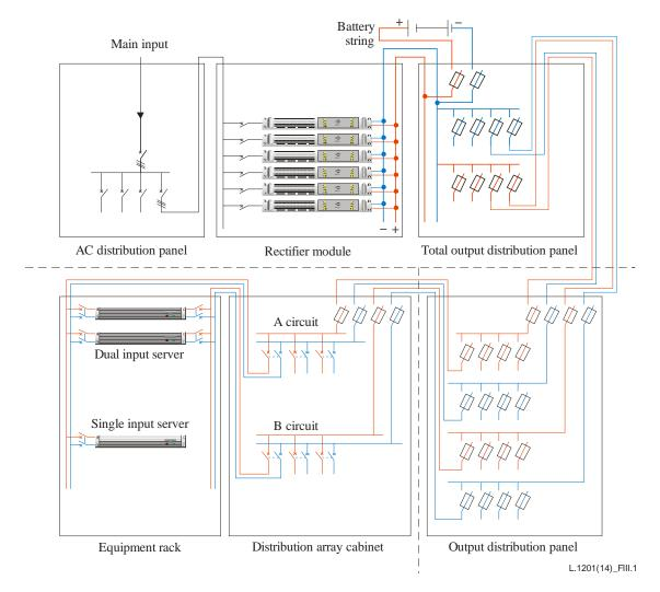
**Figure III.1 – Three-level distribution structure**
