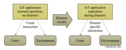
Figure 1 – Operation mode change for IoT applications with dedicated operation mode activated during disaster
