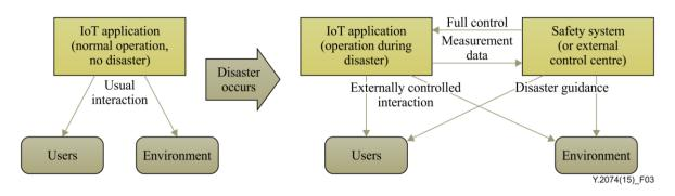
Figure 3 – Operation mode change for IoT applications with external control of operation during disaster
