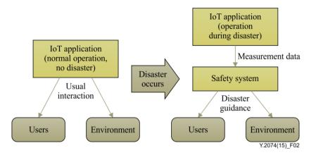
Figure 2 – Operation mode change for IoT applications temporally providing resources to external safety systems during disaster
