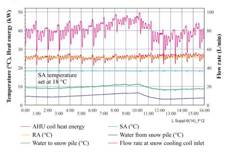
Figure 12 – Air temperature in snow and ice cooling
