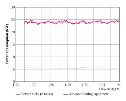
Figure 13 – Power consumption of servers and air conditioning equipment (snow and ice cooling)
