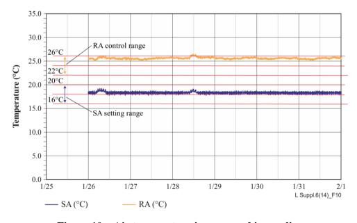
Figure 10 – Air temperature in snow and ice cooling
