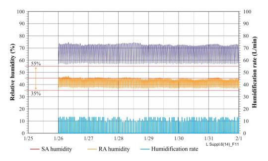
Figure 11 – Relative humidity of air and the humidification rate
