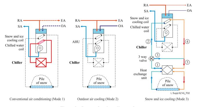
Figure 2 - Image of each cooling mode
