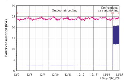
Figure 8 – Power consumption of servers and air conditioning equipment
