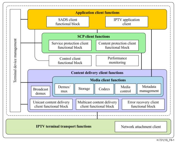
Figure 8-1 – Functional architecture block diagram of a basic model IPTV terminal device
