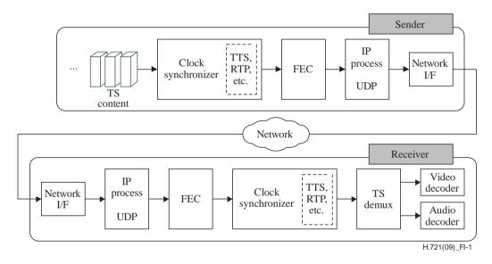
Figure I.1 – System overview of the clock synchronization
