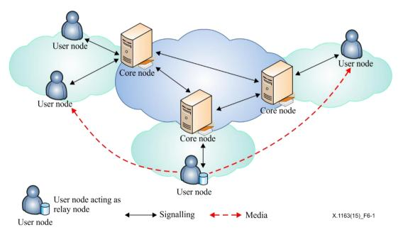
Figure 6-1 – Telecommunication network architecture based on P2P
