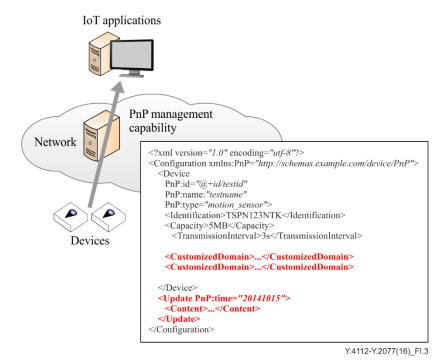
Figure I.3 – Use case of customized configuration of IoT device
