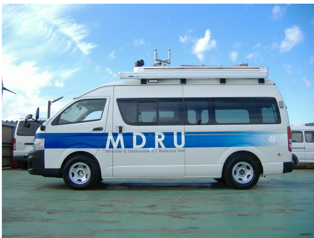
Figure I.7 – A van-type movable and deployable ICT resource unit
