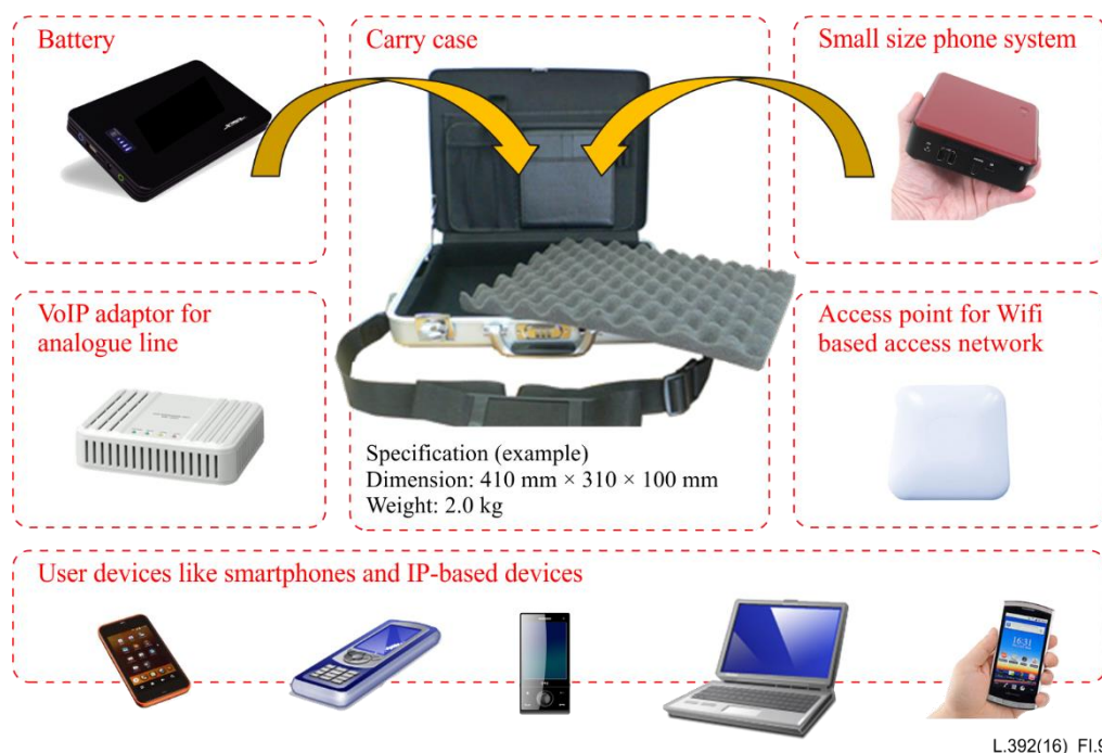
Figure I.9 – Briefcase-type movable and deployable ICT resource unit
