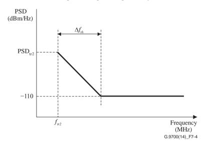
Figure 7-4 – High-frequency edge out-of-band LPM
