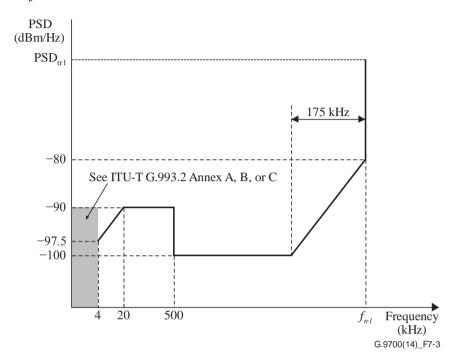
Figure 7-3 – Low-frequency edge out-of-band LPM
