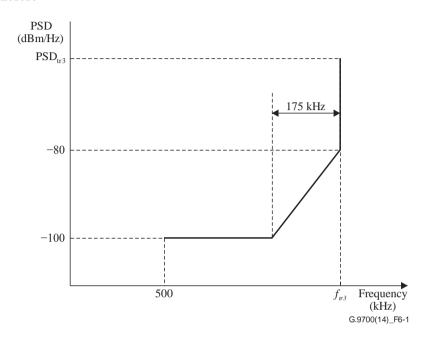
Figure 6-1 – Low-frequency edge stop-band mask
