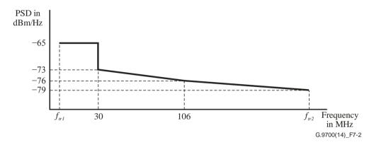
Figure 7-2 – In-band limit PSD mask for 212 MHz profile
