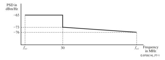
Figure 7-1 – In-band limit PSD mask for 106 MHz profile
