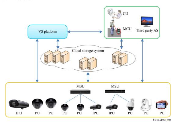
Figure 1 – Cloud storage model for visual surveillance
