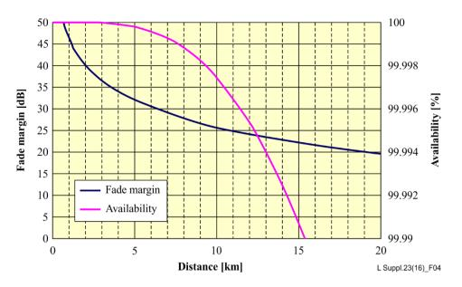
Figure 4 – Example of link budget calculation at 15 GHz: Fade margin and availability versus distance
