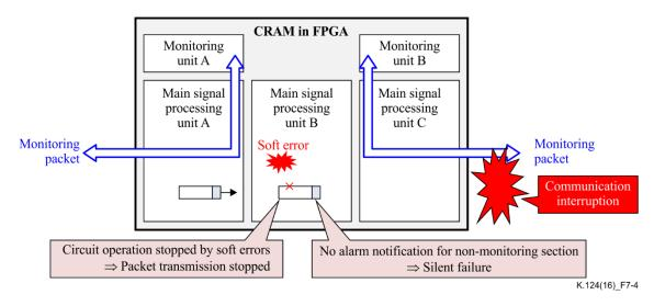
Figure 7-4 – Client signal interruption due to failure of CRAM in FPGA
