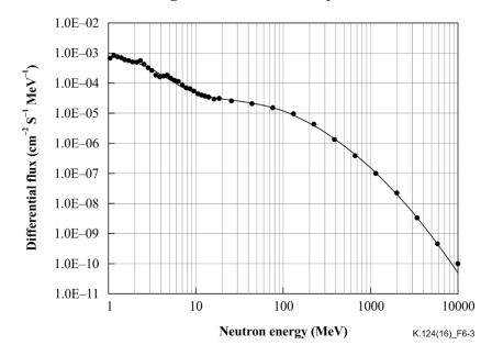
Figure 6-3 – High-energy neutron spectrum at sea level in New York City [b-JEDEC]
