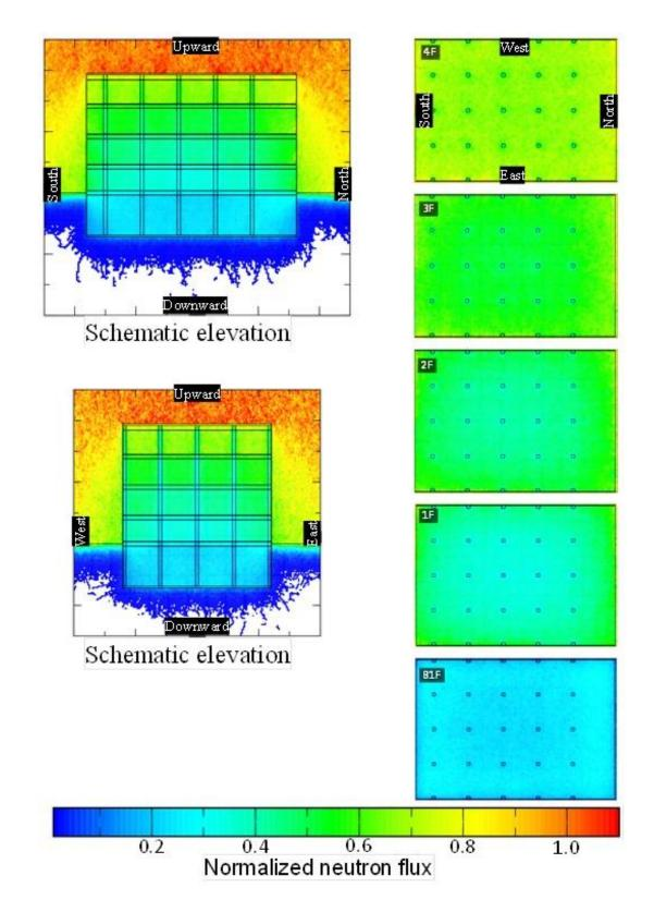
Figure 6-7 – Neutron flux in a telecommunications centre evaluated by computer simulations (Normalized by the assessment of flux outside of the building)
