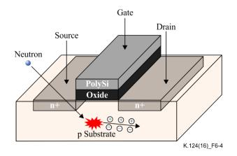
Figure 6-4 – Invasion of high-energy neutron causing soft errors
