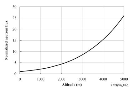
Figure 6-5 – Neutron flux variation with altitude
