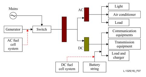
Figure 7 – Hydrogen fuel cell-powered system DC power supply and AC power lines
