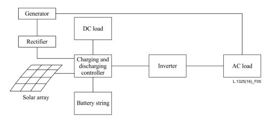
Figure 5 – Solar and DG power system
