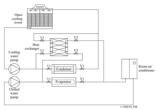
Figure 8 – Open cooling tower cooling system
