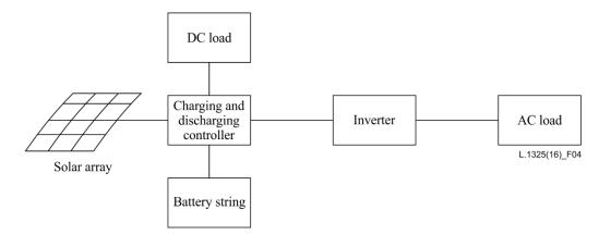
Figure 4 – Off-grid solar power system
