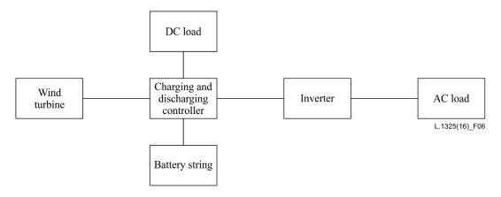
Figure 6 – Off-grid wind power system structure
