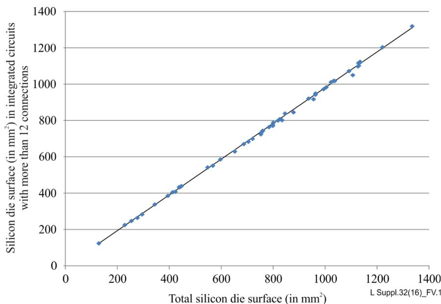
**Figure V.1 – Correlation between the silicon die area of IC chips having 12 or more pins and the total silicon die area in 50 different mobile phones**
