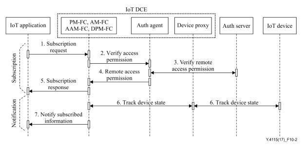
Figure 10-2 – Flow for subscribing IoT device capabilities with remote access permissions
