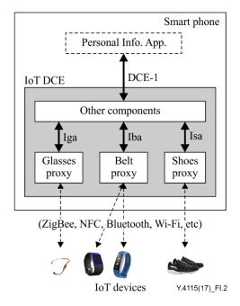
Figure I.2 – Use case of personal data integration – Case using IoT DCE
