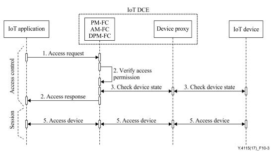
Figure 10-3 – Flow for accessing to exposed IoT device capabilities
