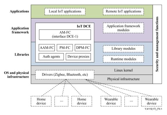
**Figure II.1 – Implementation example of IoT DCE**
