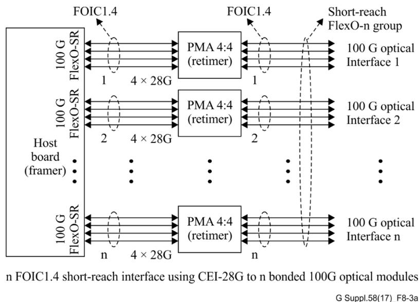
**Figure 8-3a – Original application of a FOIC1.4 interface**
