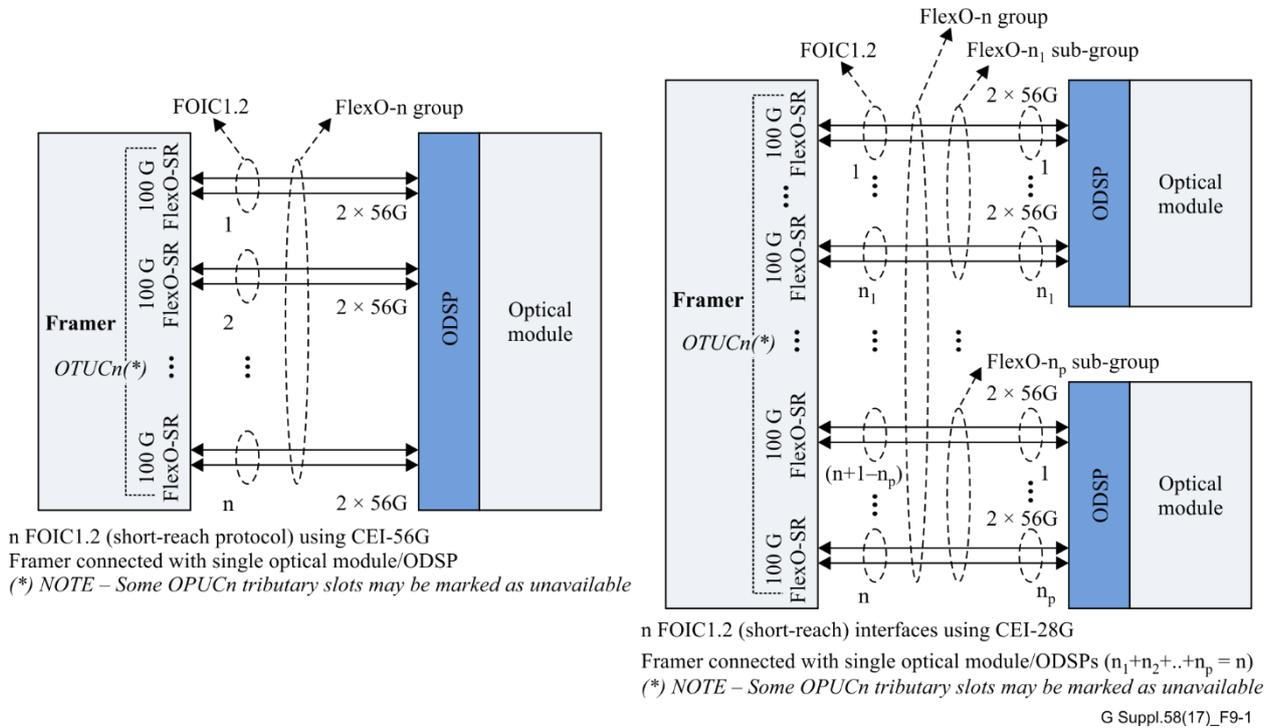
**Figure 9-1 – Example applications of a FOIC1.2 interface**
