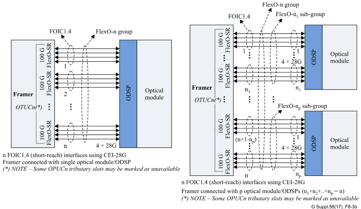
**Figure 8-3b – Alternate application of a FOIC1.4 interface**
