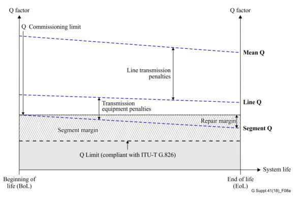
Figure 8-a – Power budget structure of example 1
