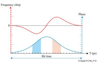
Figure 12 – Temporal variation of the phase shift and the frequency chirp induced by SPM [b-Agrawal]
