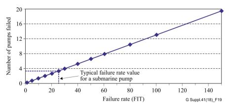
Figure 19 – Estimated number of pumps failed in 25 years for a typical transatlantic link composed of one fibre pair and 150 repeaters containing four pumps each
