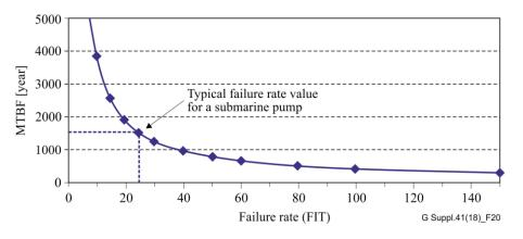
Figure 20 – MTBF for a second pump failure in the same repeater in a typical transatlantic link composed by one fibre pair and 150 repeaters with four redundant pumps each
