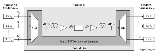
Figure 28 – Multi-span black-link transverse compatibility
