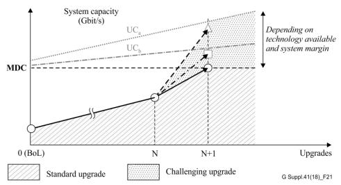
NOTE – UC<sub>a</sub> (resp. UC<sub>b</sub>) is UC when replacing (resp. keeping) the existing equipment. Note that curve UC<sub>b</sub> is deduced from curve UC<sub>a</sub> and the actual system loading. For clarity purposes, curve UC<sub>a</sub> was assumed quasi linear.
