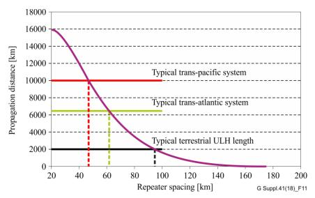
NOTE – The parameters used are: OSNR = 16 dB in a reference bandwidth  $B_r = 0.1$  nm, NF = 4.7 dB,  $N_{\lambda} = 64$  channels,  $P_{out} = 14$  dBm and fibre attenuation  $\alpha = 0.21$  dB/km.
