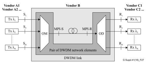
Figure 27 – Single-span black-link transverse compatibility
