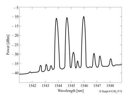
Figure 13 – Optical power spectrum measured at the output of 25 km length of dispersion shifted ( $D = -0.2 \text{ ps/nm} \cdot \text{km}$  at the central channel) when 3 mW channels are used [b-Tkach]
