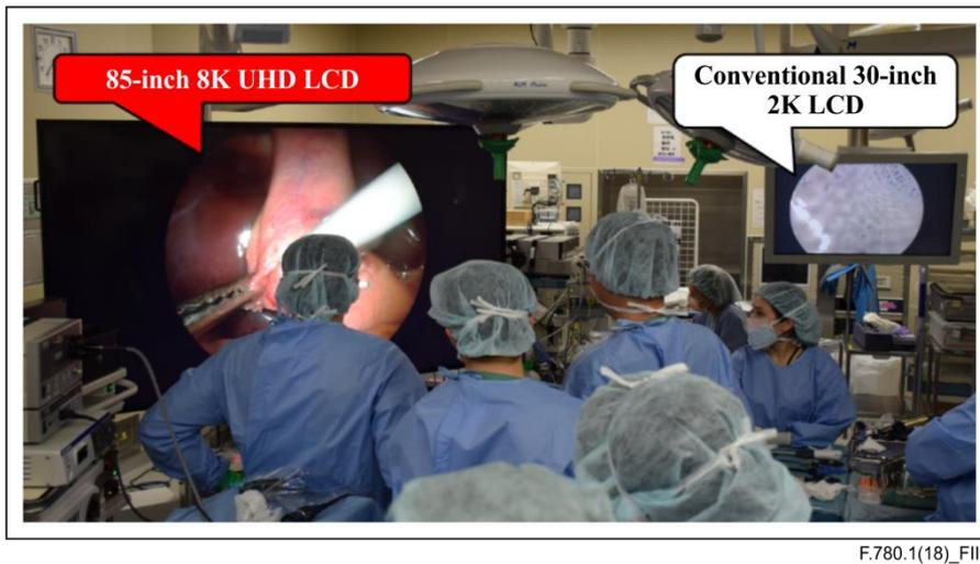
**Figure II.8 – Surgeon's view of 8K UHD LCD in the operation room**
