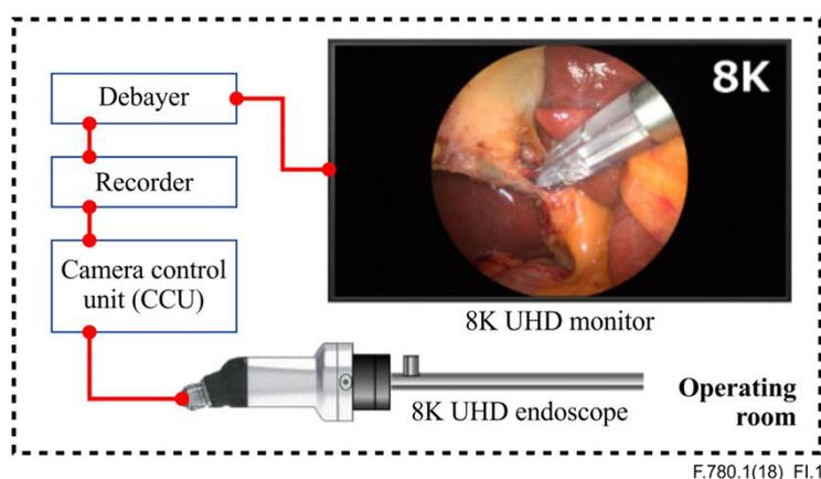
**Figure I.1 – 8K endoscope system with real-time recorder**
