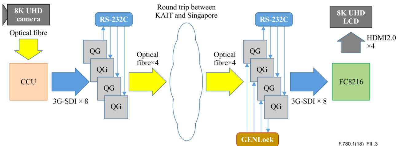
**Figure III.3 – Connection between 8K UHD camera and 8K UHD LCD by way of round trip between Japan (KAIT) and Singapore**
