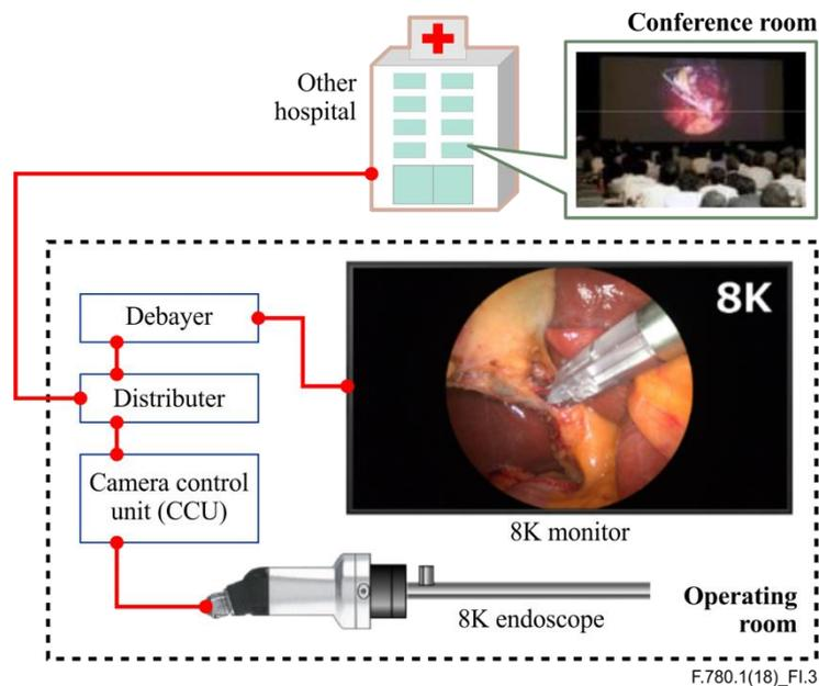
**Figure I.3 – 8K endoscope system with teleconference (remote site)**
