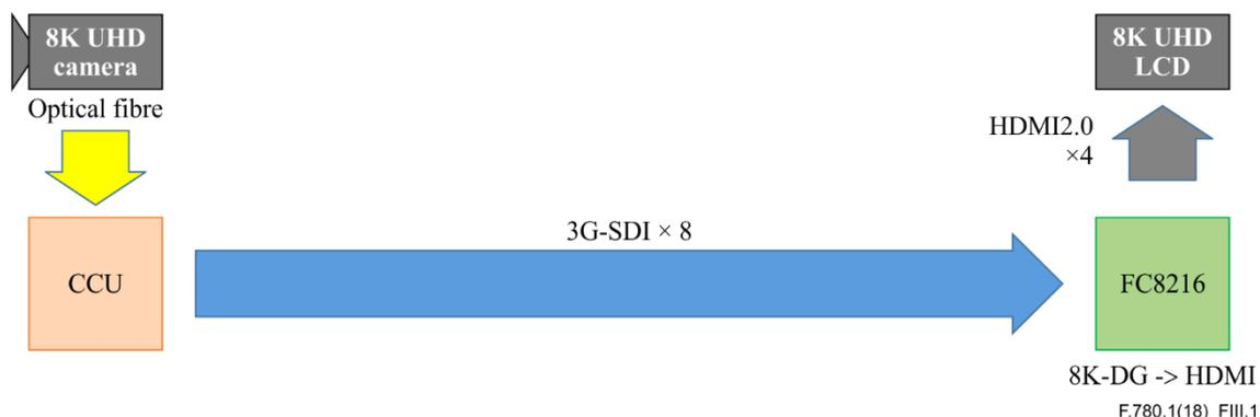
Figure III.1 – Local connection between 8K UHD camera and 8K UHD LCD
