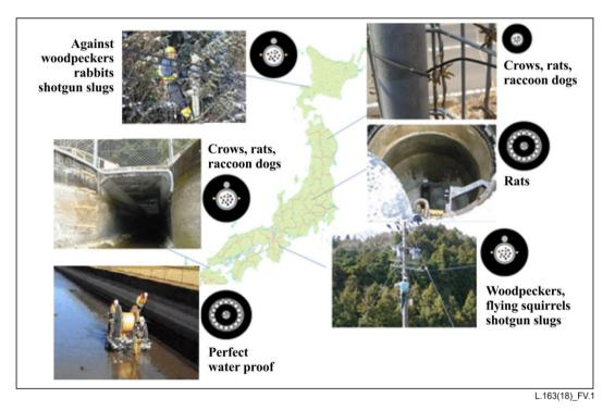
Figure V.1 – DSA cables implemented in Japan between 2000-2016
