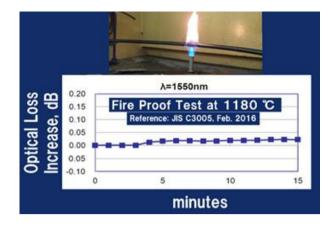
Figure V.4 – Fire proof test of a DSA cable
