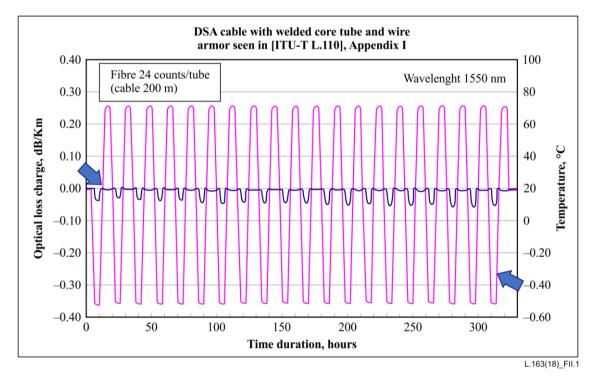
Figure II.1 – Example of optical loss changes of a DSA cable against heat cycle
