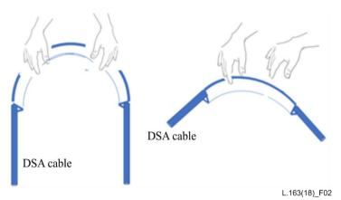
Figure 2 – A bend protector concept for safe handling of the DSA cable
