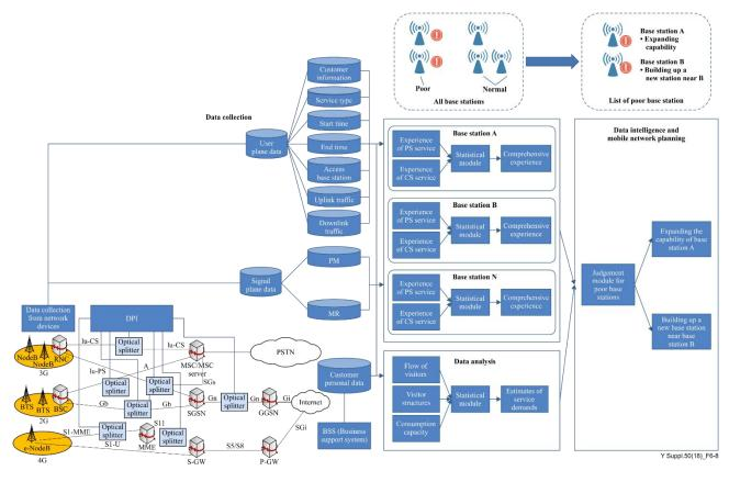
Figure 6-8 – Big-data-driven mobile network planning and construction based on customer experience
