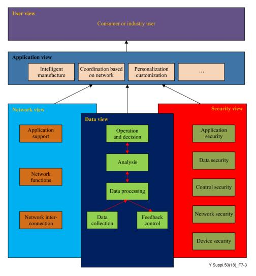
Figure 7-3 – Example reference architecture for the industrial Internet
