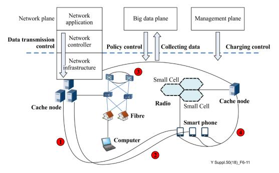
Figure 6-11 – Content transmission control to the content delivery network end user in big-data-driven networking
