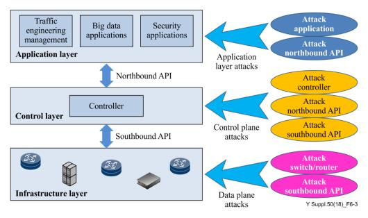
Figure 6-3 – Potential attacks on the three layers of bDDN architecture
