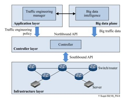
Figure 6-9 – Dynamic traffic engineering system architecture with software-defined networking and big data
