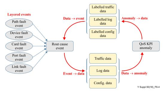
Figure 6-4 – Big-data-driven quality of service anomaly detection and root cause tracking
