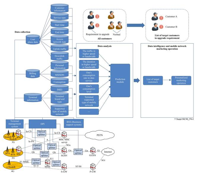
Figure 6-2 – Big-data-driven prediction of customer upgrade in mobile network
