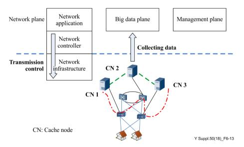
Figure 6-13 – Content transmission control between the content delivery network cache nodes in big-data-driven networking
