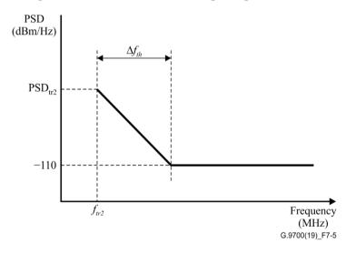
Figure 7-5 – High-frequency edge out-of-band LPM to be used in combination with LPM\_106 and LPM\_212
