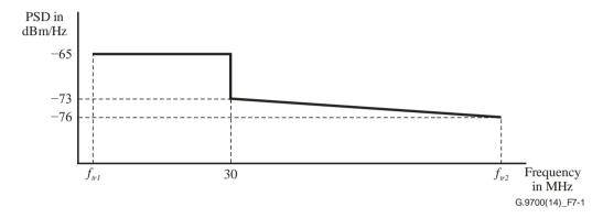
Figure 7-1 – In-band limit PSD mask LPM\_106
