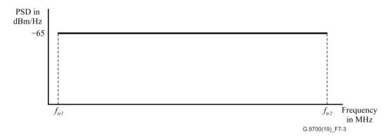
Figure 7-3 – In-band limit PSD mask LPM\_106high
