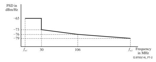
Figure 7-2 – In-band limit PSD mask LPM\_212
