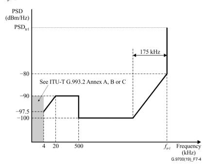
Figure 7-4 – Low-frequency edge out-of-band LPM
