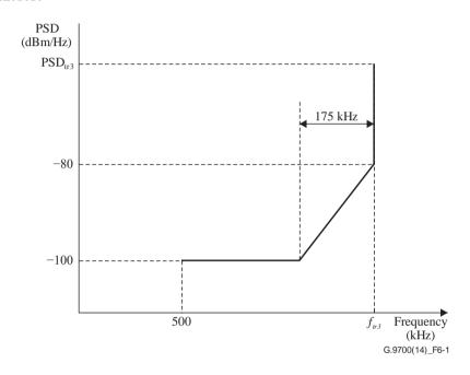
Figure 6-1 – Low-frequency edge stop-band mask
