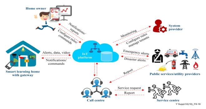
Figure 8-18 – Home automation system process flow
