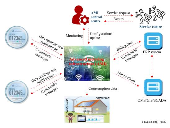
Figure 8-20 – Process flow diagram
