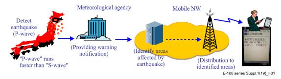
Figure 1 – Tsunami Mobile Early Warning System Japan
