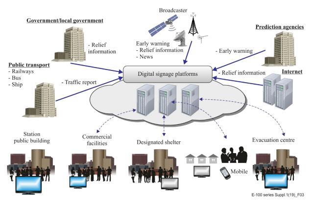
Figure 3 – Digital signage system for disaster relief and early warning
