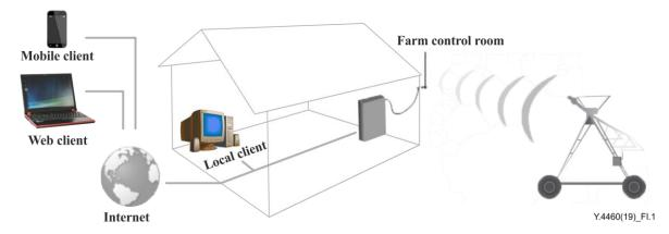
Figure I.1 – Irrigation monitoring system using LPLC architectural reference model
