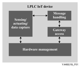
Figure 1 – Architectural reference model for LPLC devices
