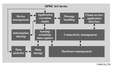
Figure 3 – Architectural reference model for HPHC devices
