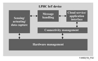
Figure 2 – Architectural reference model for LPHC devices
