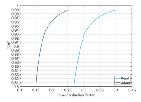
Figure 7 – Cumulative distribution functions (CDFs) of the power reduction factor for rural and urban installation scenarios of an 8x8 massive MIMO antenna array
