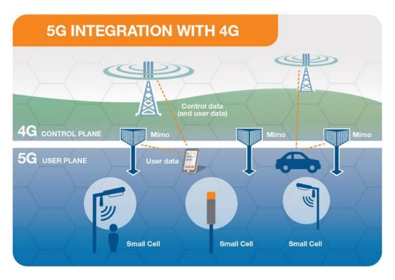
Figure 5 – How the 5G networks will initially be integrated with existing 4G networks [b-EmfExpl]
