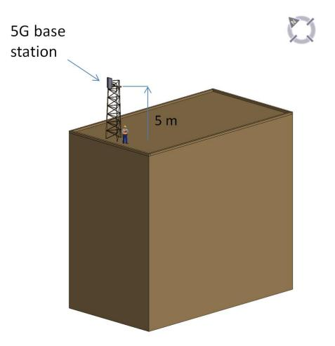
Figure 6 – Drawing of the assessed 5G macro site with a 3.5 GHz massive MIMO base station. The lower part of the antenna is at a 5-metre height above the rooftop [b-EmfExpl]
