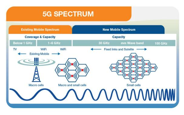
Figure 1 – Existing and new spectrum to be used for 5G mobile communication services [b-EmfExpl]
