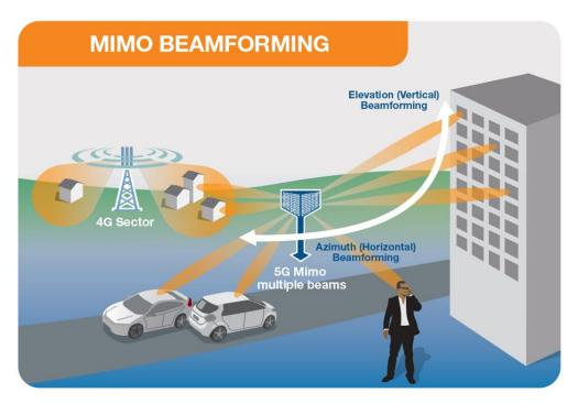
Figure 4 –Massive MIMO beamforming and beam steering in a 5G network [b-EmfExpl]
