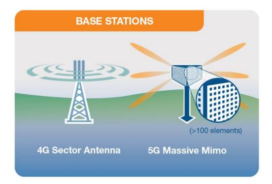
Figure 3 – 4G base station with sector antennas and 5G base station with multi-element massive MIMO antenna array [b-EmfExpl]
