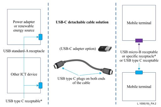
\* In the case of a specific connector on the mobile terminal, the adapter between micro USB plug and the device receptacles is not represented on the figure
