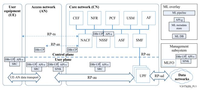
Figure I.1 – Example of realization in an IMT-2020 network
