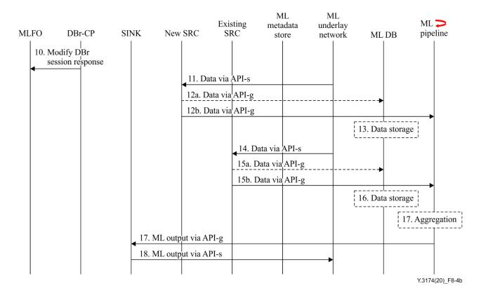
Figure 8-4-b – Addition of new SRC in data handling framework (part b)
