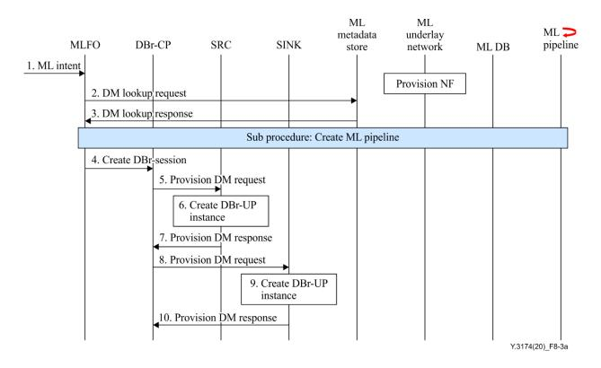
Figure 8-3-a – Instantiation of a data handling framework (part a)
