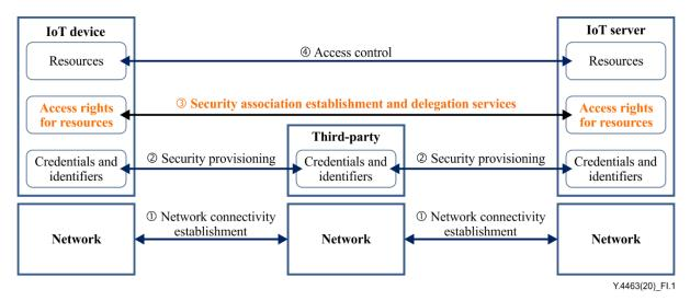
Figure I.1 – Four security phases of IoT devices
