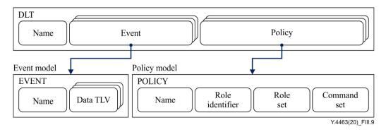
Figure III.9 – Data model for distributed database
