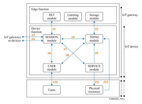
Figure III.2 – Interfaces of IoT gateways and devices
