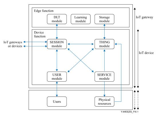
Figure III.1 – Core functions in IoT gateways and devices
