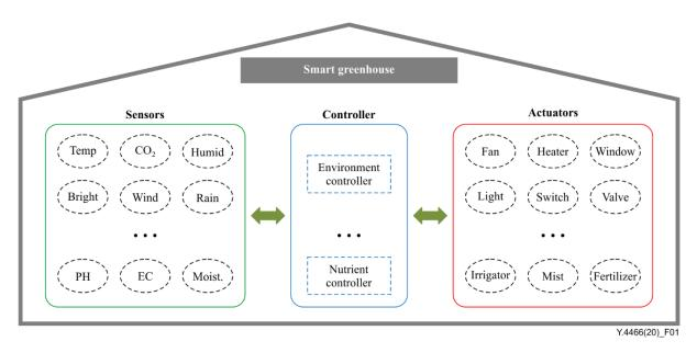
Figure 1 – Conceptual diagram of smart greenhouse
