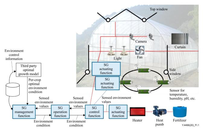
Figure I.1 – Smart greenhouse use case
