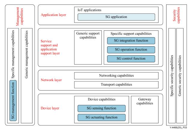
Figure 3 – SG service reference model in accordance with the IoT reference model [ITU-T Y.4000]
