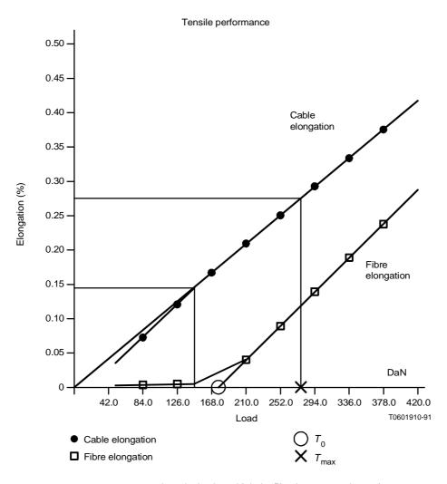
Note  $-T_0$  corresponds to the load at which the fibre becomes under strain.  $T_{\text{max}}$  corresponds to the maximum specified pulling load.
