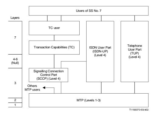
FIGURE 2/Q.700 Architecture of SS No. 7
