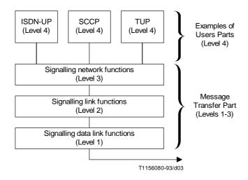
FIGURE 3/Q.700 SS No. 7 functional levels
