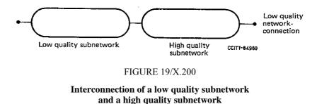
b) The lower quality subnetwork is enhanced equal to the higher quality subnetwork and the subnetworks are then interconnected. The quality of the resulting network-connection is aproximately that of the higher
