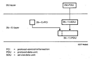
Note 1 – This figure assumes that neither segmenting nor blocking of (N)-service-data-units is performed (see § 5.7.6.5). Note 2 – This figure does not imply any positional relationship between protocol-control-information and user-data in protocol-data-units. Note 3 – An (N)-protocol-data-unit may be mapped one-to-one into an (N-1)-service-data-unit, but other relationships are possible (see Figure 11/X.200).
