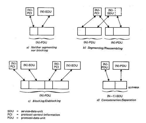
Note 1 - This figure does not imply any positional relationship between protocol-control-information and user-data in protocol-data-units. Note 2 - In the case of concatenation, (N)-protocol-data-unit does not necessarily include an (N)-service-data-unit.
