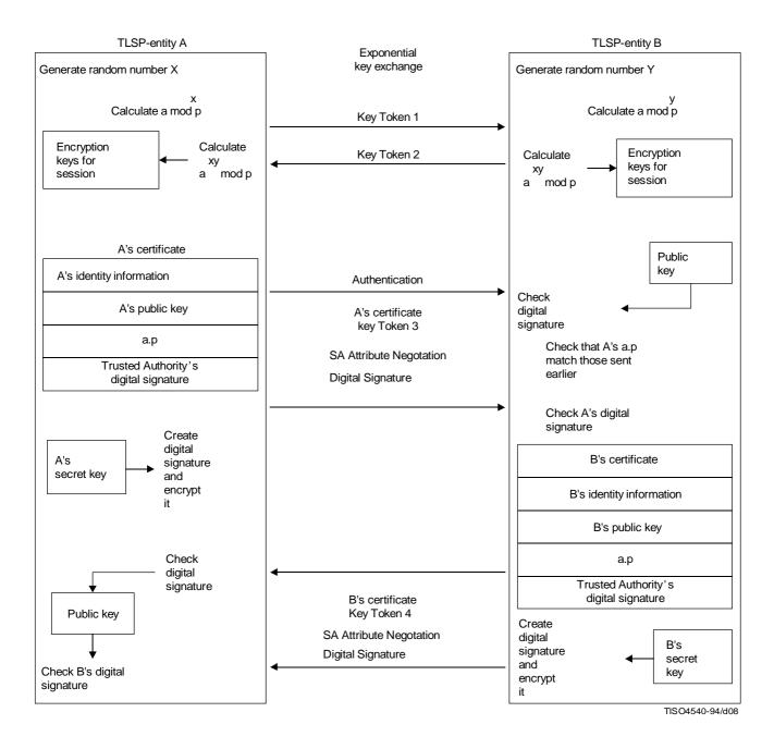
Figure D.1 – Illustration of On-Line Key Derivation and Digital Signature using EKE
